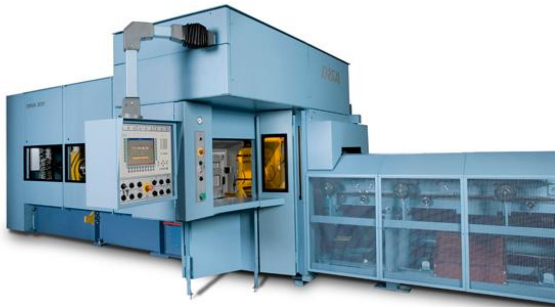
Figure 3.1 The DISAMATIC - DISA's sand moulding machine
